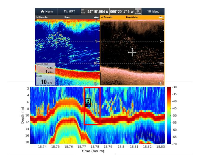
Figure 22: (Top) Fish school observed using the Puffin's Raymarine echosounder in Grand Passage, August 26, 2019. (Bottom) Backscatter intensity data, in dB re  $1 \text{ m}^{-1}$ , from beam 1 of the Nortek Signature500 ADCP deployed aboard the Puffin. The red box corresponds to the time and space intervals shown in the Raymarine echogram. Fish velocity estimates were computed using a subset of the fish school, shown by the black box. Detected fish are indicated by black dots.
