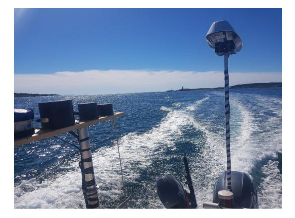
Figure 3: Vessel-mount configuration aboard the RV Puffin in Grand Passage. The four instruments on the pole mount (left of image) from left to right are the 600 kHz RDI ADCP and the 38 kHz, 120 kHz, and 200 kHz BioSonics DTX transducer heads. The post on the right is a GPS receiver.
