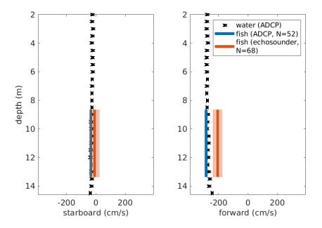
Figure 20: Selected fish school 1: Current velocity profiles for the the across-vessel (left) and along-vessel (right) components of velocity. The mean fish school velocities from the ADCP and echosounder, with 95% confidence intervals, are indicated by the coloured vertical lines and shaded boxes.
