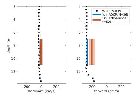
Figure 21: Selected fish school 2: Current velocity profiles for the the across-vessel (left) and along-vessel (right) components of velocity. The mean fish school velocities from the ADCP and echosounder, with 95% confidence intervals, are indicated by the coloured vertical lines and shaded boxes.
