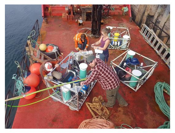
Figure 4: Bottom frame being prepared for deployment in Grand Passage, 2018.
