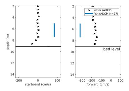
Figure 23: Current velocity profiles for the the across-vessel (left) and along-vessel (right) components of velocity, computed using data from a Nortek Signature500 ADCP (no corresponding split-beam echosounder data). The mean fish school velocities from the ADCP are indicated by the blue vertical lines.
