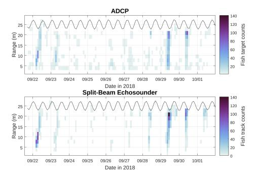
Figure 13: Time series of fish target counts from the ADCP (upper) and sigle echo detection track counts from the split-beam echosounder (lower). Figure from *Dunn* (2019).
