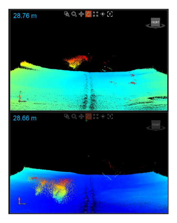
Figure 10: Sidescan sonar images from the Jetyak-mounted Ping DSP sonar, September 1, 2020. Returns from a fish school are visible (red-yellow-green). The water depths at times of recording were 28.76 m and 28.66 m.
